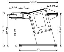
Sterling Modular Systems,inc 704 East 4th Street, Boyertown PA 19512 610-369-5802 www.sterlingmodular.com The "Controller" version of the Multi-Station is configured for the small footprint keyboards that are 10 1/2" deep (or less).
